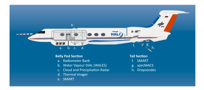
HALO is configured to function as an airborne cloud observatory with a great variety of remotesensing instruments on board along with a dropsonde launching system. For greater detail, refer to Stevens et al (2019). The instruments have been listed in the table below.
