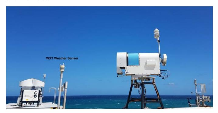
It provides 6 of the most important weather parameters: air pressure, temperature, humidity, rainfall, wind speed and direction on approx. 4 m AGL. The data is recorded every 10 seconds (10s mean values from 1s values).
