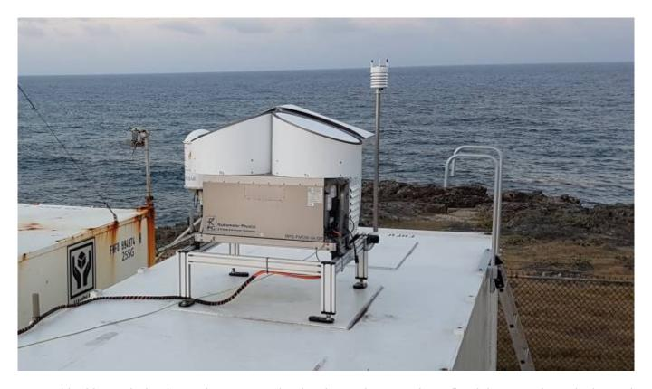
Upward looking polarized Doppler 94 GHz cloud radar to detect radar reflectivity, Doppler velocity and linear depolarization ratio of cloud particles. The W-Band radar is measuring since December 2018 at altitudes between 150 m and 15 km with a temporal resolution of 2 s.
